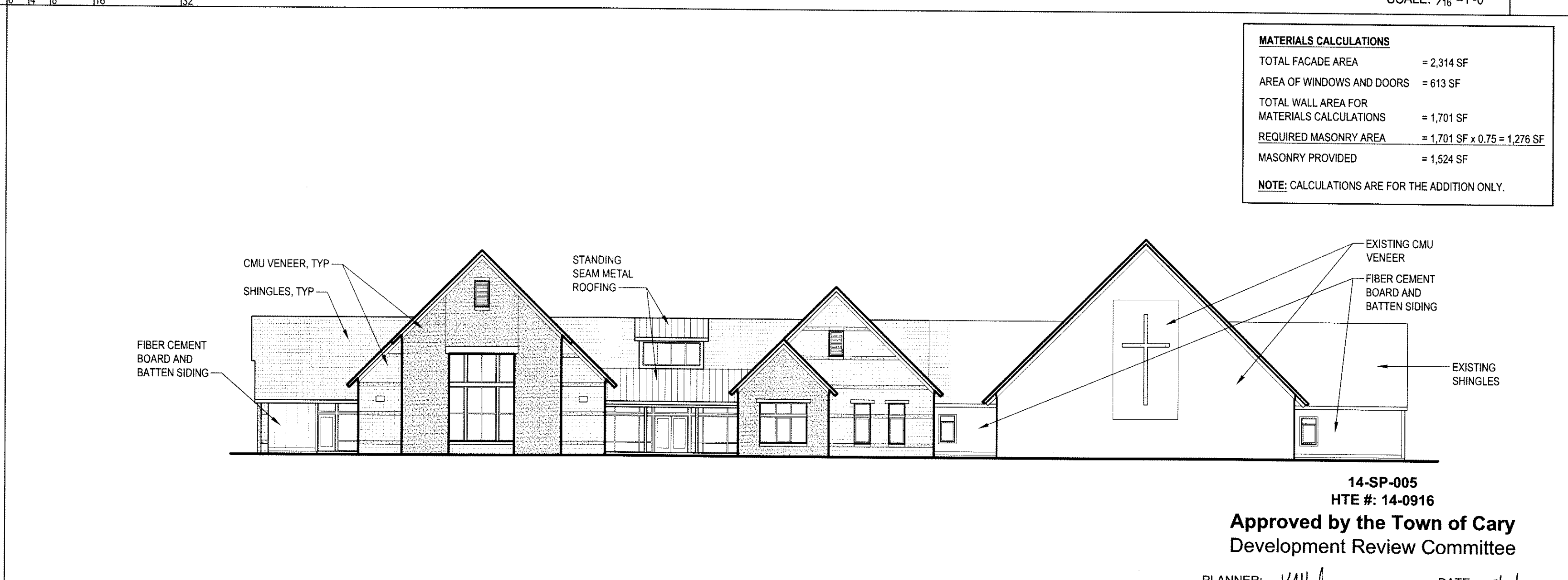
SOUTH ELEVATION - MATERIALS OVERLAY
