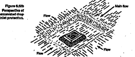
Figure 6.50b: Perspective view of excavated drop inlet protection.
